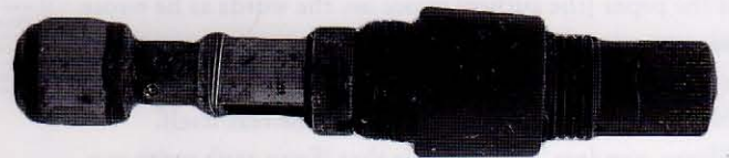
Montblanc Internal spiral threads and repaired filler.
